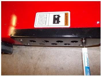
For both left and right sides, slightly unscrew side panels and slide off.
