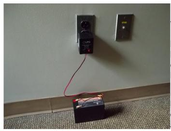
Finally, for both batteries, plug the battery to the charger by the yellow connector. Expected charge time for one battery is 8 hours. When done charging both batteries, reattach batteries to robot and close side panels. Please recharge batteries after every 8 hours of use.
