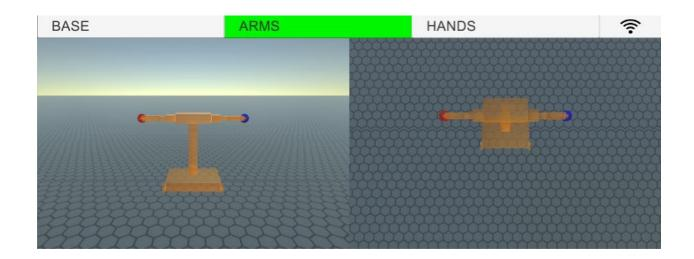
The window contains three tabs: one for controlling the base, one for the arms and one for the hand grippers.
